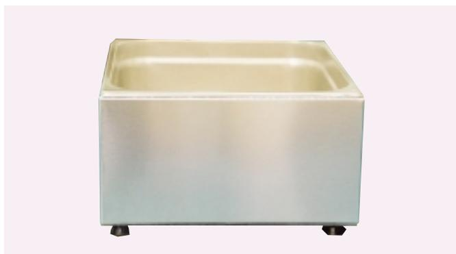
Metallic tanks in stainless steel, double external body in stainless steel AISI-304 and interior in stainless steel 18//10, aisled with polyurethane foam, adequate to work with cooling units to avoid condensation.
